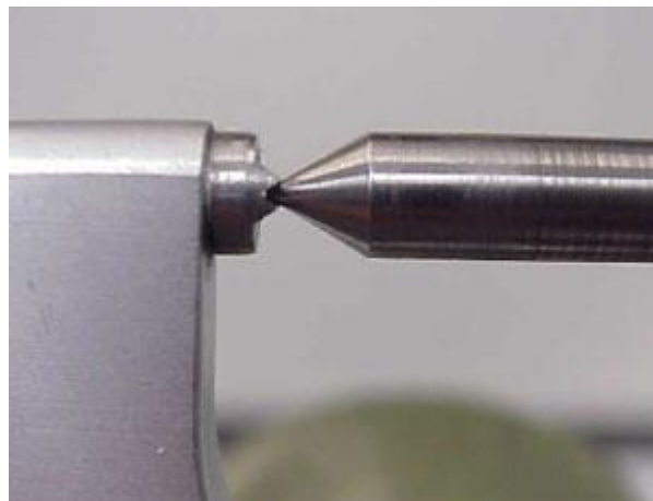
Fig. The pitch line indicates the imaginary thread profile engagement.
