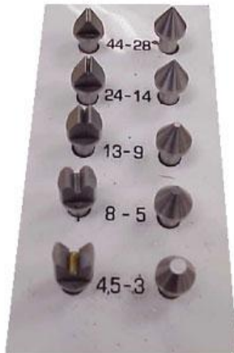
Fig. Set of interchangeable anvils for an interchangeable anvil screw thread micrometer
