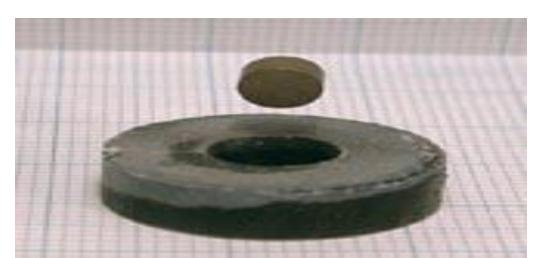
➤ By surrounding a diamagnetic material with a magnetic field, it can be held in a stationary position (the magnetic force is strong enough to counteract gravity.)
