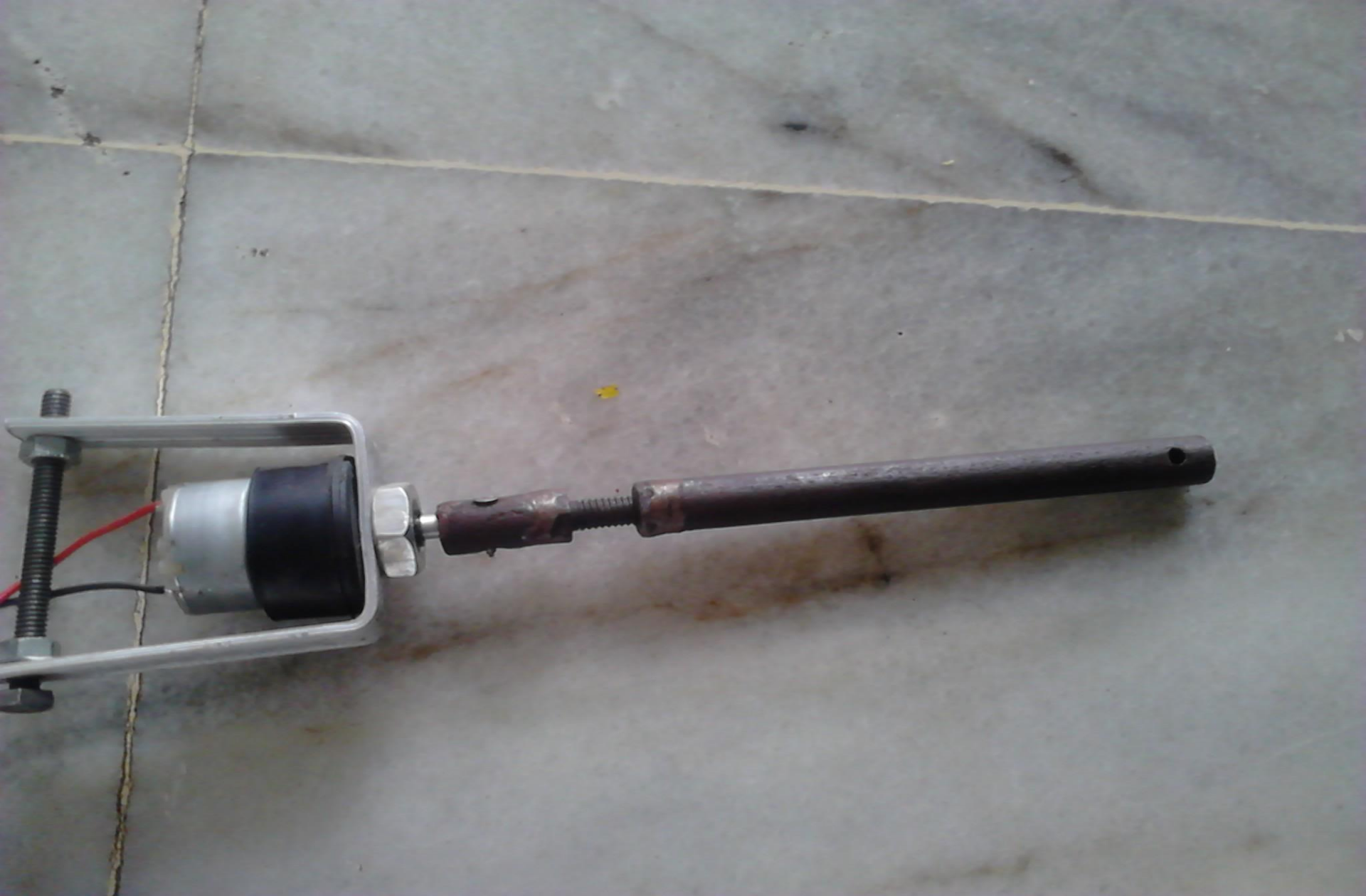
150 R.P.M. MOTOR CONNECTED WITH ACTUATOR
