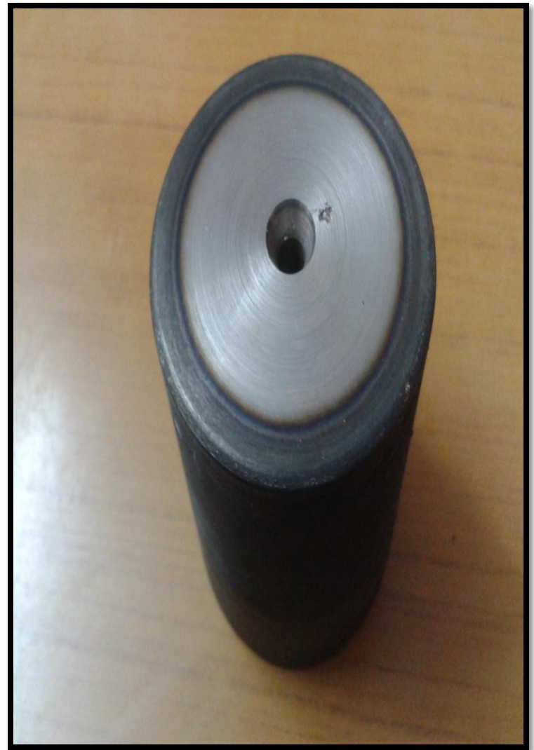
Fig-11 Induction Hardening EN41B specimen
