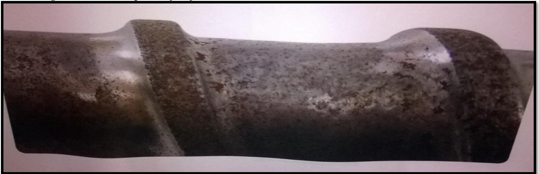
Fig- 4 corrosion part of injection screw. [15]
