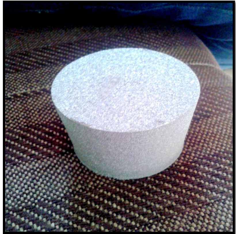
Fig-13 WC coating EN41B specimen
