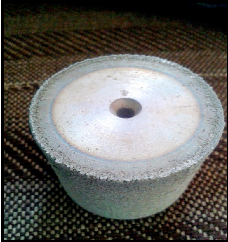
Fig-12 Induction Hardening and WC coating EN41B specimen
