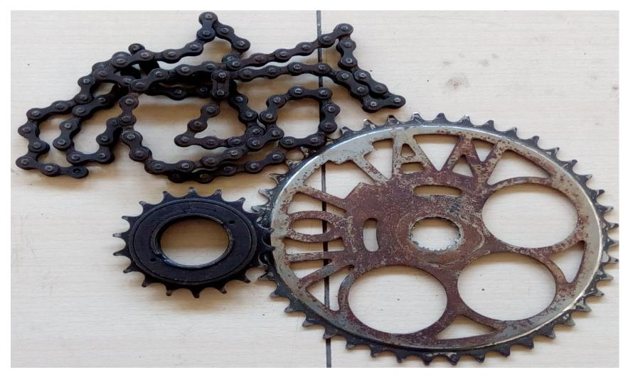
Big chucker teeth=44 Small chucker teeth=18 Gear ratio=2.44
