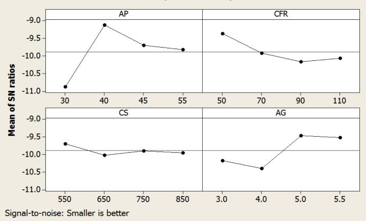
Fig. shows that the lower KW will meet at air pressure 30 N/cm<sup>2</sup>, current flow rate 90 A, cutting speed 650 mm/min and arc gap 4 mm. The graph generate by the use of MINITAB statistical software for KW.
