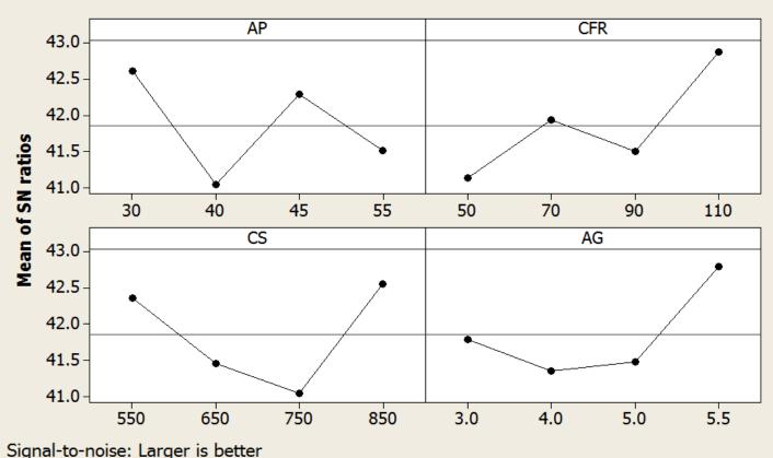
Fig. shows that the higher MRR will meet at air pressure 30 N/cm<sup>2</sup>, current flow rate 110 A, cutting speed 850 mm/min and arc gap 5.5 mm. The graph generate by the use of MINITAB statistical software for MRR.
