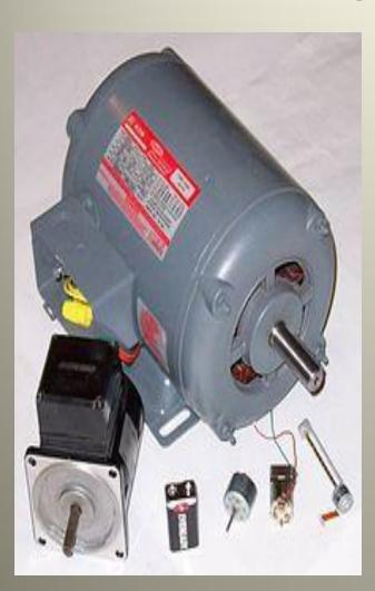
an electric motor is an electrical machine that converts electrical energy into mechanical energy.
